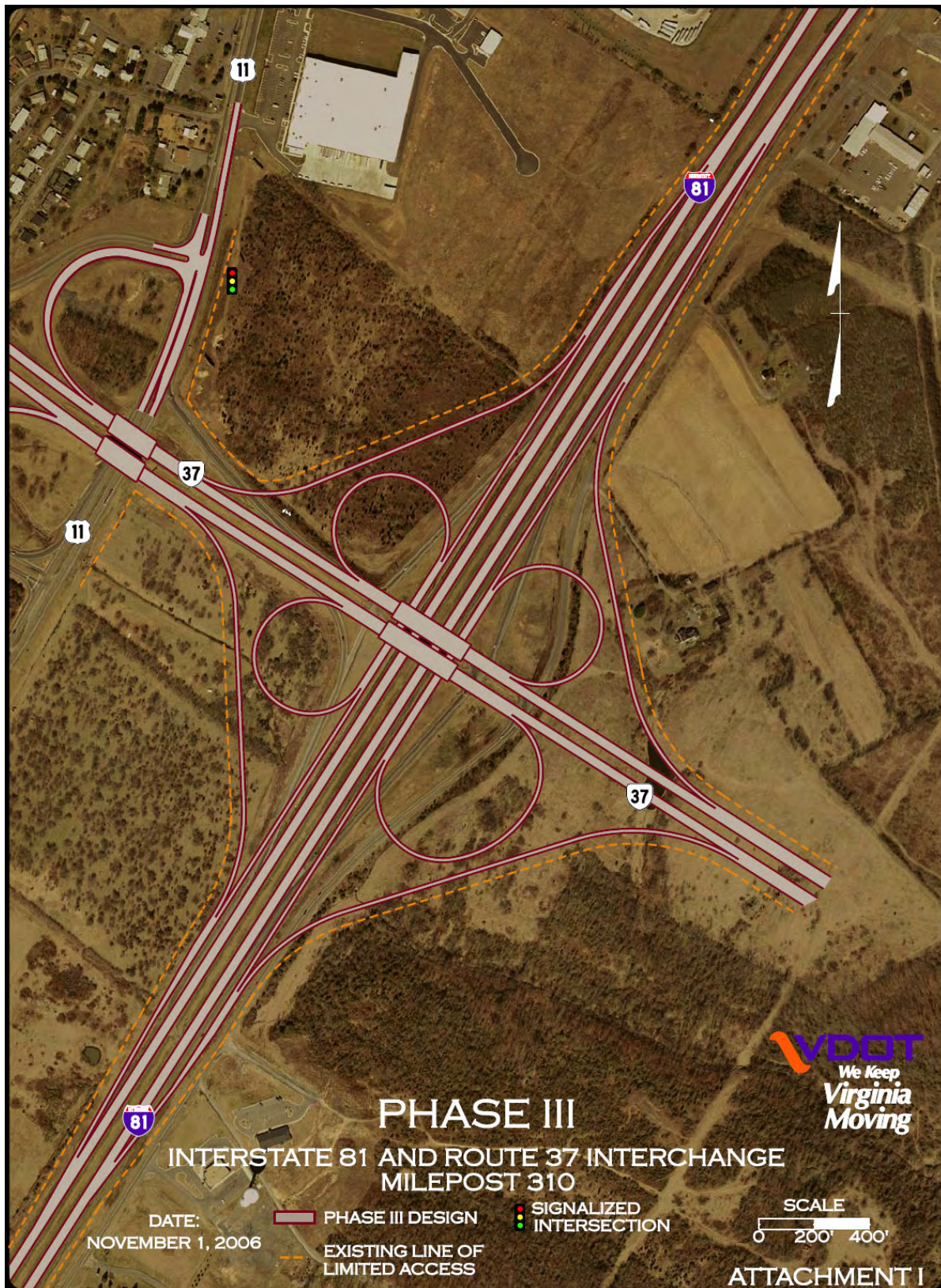
Figure 3: Planned Interchange Improvements at I-81/Route 37 - Ultimate Configuration
