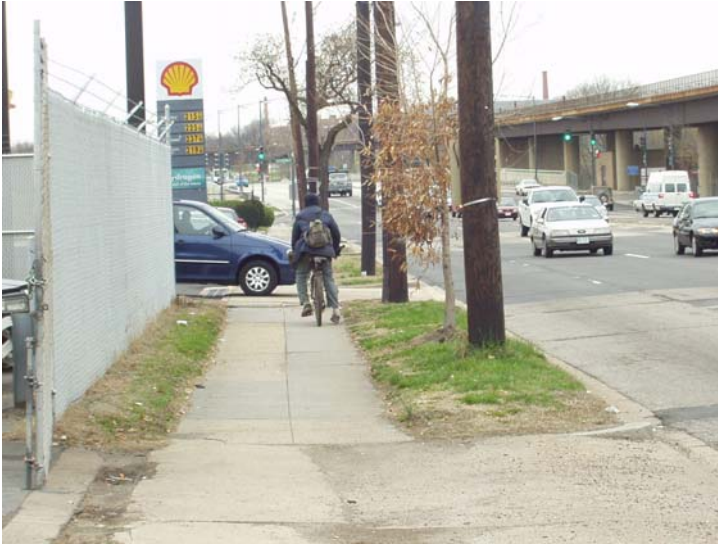
Driveways and intersections create conflicts between bicyclists on sidepaths/sidewalks and motor vehicles
